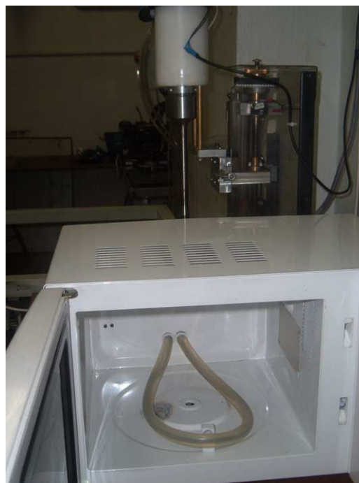
Figure 3. Reactor prototype featuring combined US/MW irradiation.
