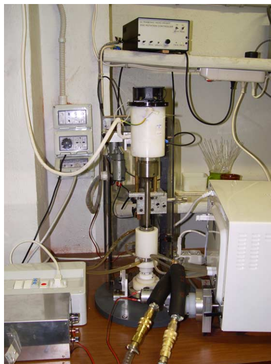
Figure 2. Reactor prototype featuring combined US/MW irradiation.
